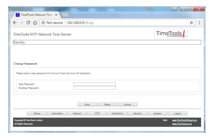
The security configuration web page allows the default HTTP, HTTPS, FTP, SSH/SCP/SFTP and console password to be modified. (Default 'admin'). A password of at least 5 characters must be entered, with a maximum of 30 characters.
