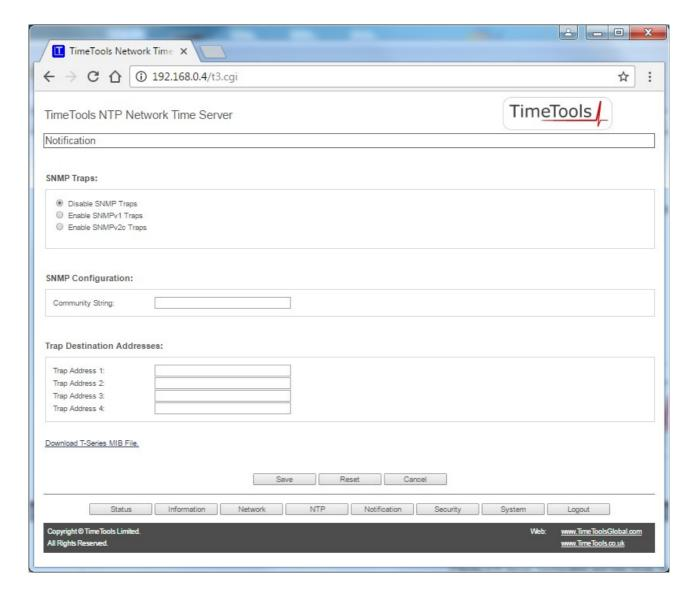
The Notification Configuration menu is used to enable and configure Simple Network Management Protocol (SNMP) traps or notifications. SNMP notifications can be used by the NTP server to warn a manager of error conditions that have occurred, such as loss of GPS signal or loss of synchronisation.
