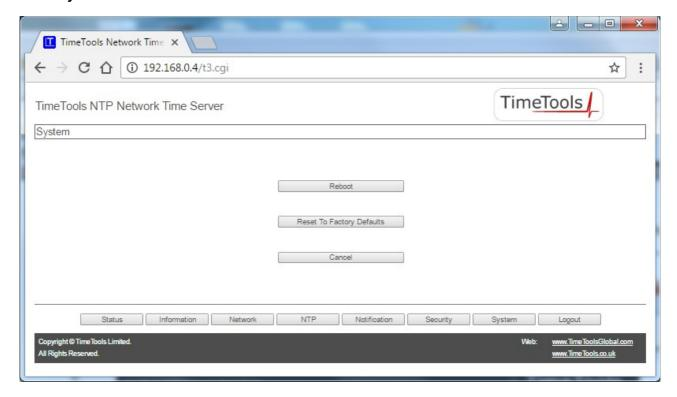
Reboot The reboot option restarts the time server. It is used to make any network configuration changes
