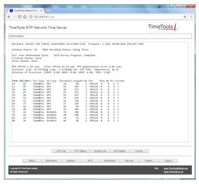
The information provided can be very useful for system debugging and installation, to find the optimum location for a GPS\GNSS antenna and to confirm signal reception levels for existing installations.
