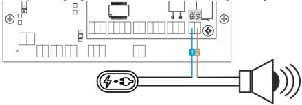
fig. 8 Buzzer and clock wiring diagram
