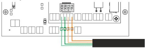
Fig. 3 LAN and clock wiring diagram
