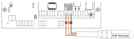
fig. 7 Temperature probe and clock wiring diagram
