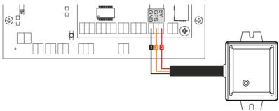
fig. 6 Connection the GPS module to the clock
