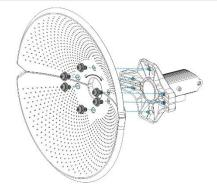
(3) Attach the antenna mounting bracket to the supporting piece using the long screw and the nut.
