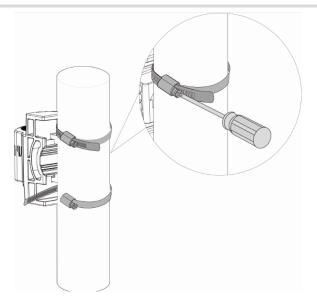
(6) Mount the assembled wireless bridge to the pole mounting bracket and tighten the long screw.
