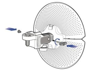
(4) Attach the wireless bridge to the front of the assembled reflectors.
