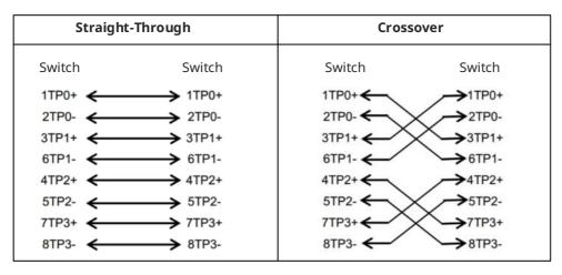
100BASE-TX/10BASE-T can be interconnected using cables of the preceding specifications. For 10 Mbps, the 100BASE-TX/10BASE-T port can be connected using 100-ohm Category 3, Category 4, and Category 5 cables; for 100 Mbps, the 100BASE-TX/10BASE-T port can be connected using 100-ohm Category 5 cables with a maximum connection distance of 100 meters. The following table shows 100BASE-TX/10BASE-T pin assignments.
