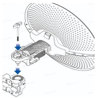
(7) Properly connect the Ethernet cable, and then install the waterproof cover. The installation is complete.
