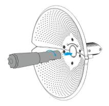
(5) Mount the pole mounting bracket to the pole, and tighten the clamps.
