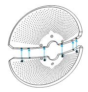
(2) Attach the supporting piece to the back of the assembled reflectors using six screws.
