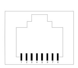
RJ45 LAN port: Connects to cameras, switches, PCs and other devices.
