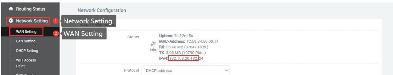
Access the internal port of the connected device through 192.168.20.132:500.(Note: The computer needs to be in the same local area network as the IP of the wan port before it can be accessed)
