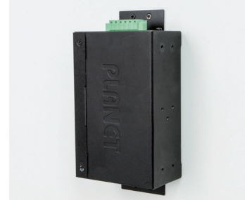
Side Wall Mounting (Space saving)
