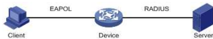
Figure 1 1 . Architecture of the 802.1X authentication system
