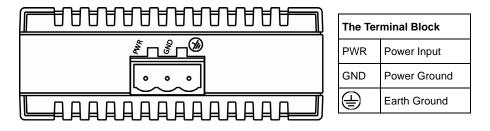
DC Terminal Block Power Input: The DC Terminal Block power input can be used to power up this Switch / Media Converter.
