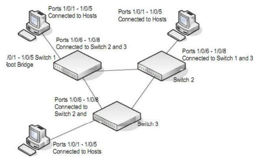
Figure 2. MSTP sample configuration
