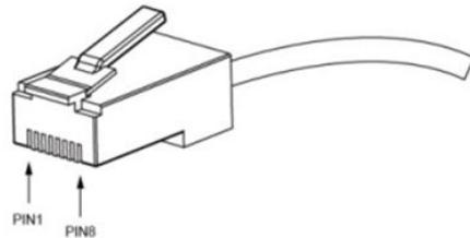
This cable is used to connect the console port of the switch to the external monitoring terminal. One end of the RJ45 eight-pin plug, the other end is a 25-hole plug(DB25) and 9-hole plug(DB9), RJ45 head into the switch's console port socket, DB25 and DB9 can be used according to the requirements of the terminal serial port, the cable internal connection schematic as follows:
