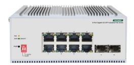
20117399 is an industrial grade Unmanaged PoE Switch 20117399 has 8\* 10/100/1000Mbps adaptive RJ45 ports and 2\*1000Mbps SFP fiber module slots. Ports 1-8 RJ45 support PoE power supply, with a maximum of 30W for each port. Each RJ45 port supports MDI/MDIX automatic rollover and wire speed forwarding.
